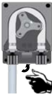
Step 18 Tighten the nut on the dosing pump.
