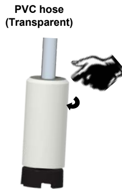
Step 16 Tighten the nut on the cone.
